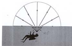
Fig. 3.7B The optical manhole. Light from the horizon (angle of incidence = 90°) is refracted downward at an angle of 48.6°. This compresses the sky into a circle with a diameter of 97.2° instead of its usual 180°.
