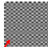
Down-sampled with a 5x5 box filter (uniform weights)
