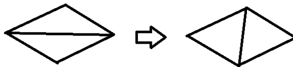
Figure 5: In this case, it improves the quality of the triangles to modify them, as shown
