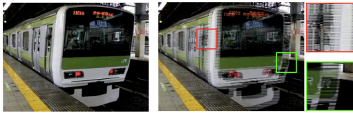
(a) Conventional rolling shutter (b) Input: interlaced readout ( K=2 )
