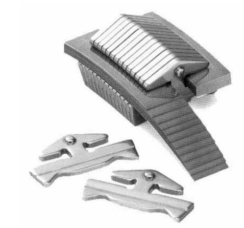
• The torque is transmitted from the input to the output pulley via friction forces between the pushbelt and the sheaves and further on via push and tension forces within the pushbelt.
