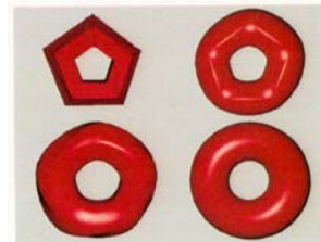
Figure 4: Interpolating a coarsely polygonized torus. Upper left: original mesh. Upper right: Shikman-Siquin interpolation[14]. Lower left: Interpolating Catmull-Clark surface. Lower right: Faired interpolating Catmull-Clark surface.
