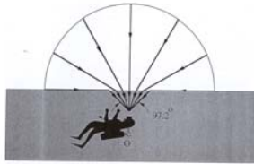
Fig. 3.7B The optical manhole. Light from the horizon (angle of incidence = 90^\circ ) is refracted downward at an angle of 48.6^\circ . This compresses the sky into a circle with a diameter of 97.2^\circ instead of its usual 180^\circ .
