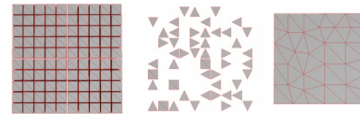
Figure 3: On the left is a regular grid of 100 closely spaced cubes. In the middle, an approximation built using only edge contractions demonstrates unacceptable fragmentation. On the right, the result of using more general pair contractions to achieve aggregation is an approximation much closer to the original.
