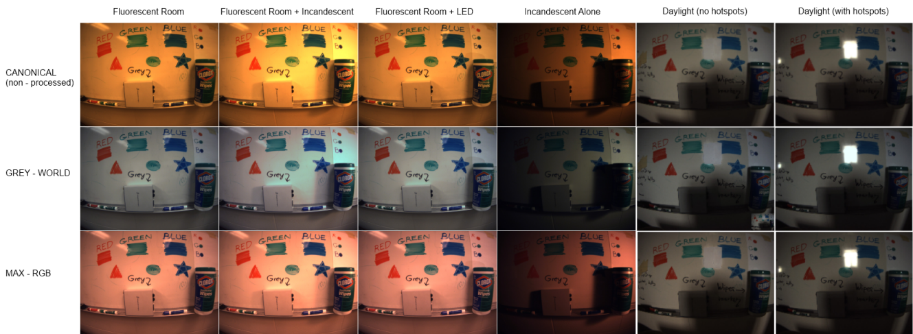
Figure 3: The Grey-World and Max-RGB color constancy algorithms, applied to input frames with lighting conditions which vary in both color and intensity.
