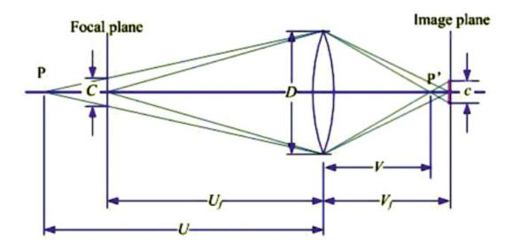
When the aperature diameter of the lens, D, is increased the amount of blurring that occurs for the same distance is increased and only the objects right on the focal plane appear to be at all in focus.
