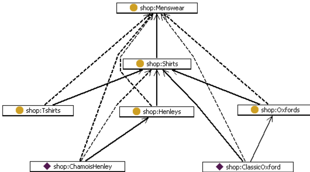
Figure 5-3. All triples in the Catalogue model. Inferred triples are shown as dashed lines.
