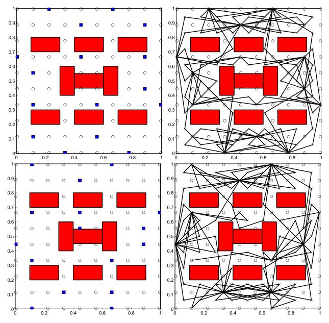
Fig. 8. **TOP ROW:** Placement obtained from the ILP solution. The figure on the left shows the selected cameras whereas the right figure shows the assignment of points (represented by  $\times$  symbols) in the workspace to the placed cameras. **BOTTOM ROW:** Placement obtained from the approximation algorithm. In this simulation, both algorithms place 16 sensors.
