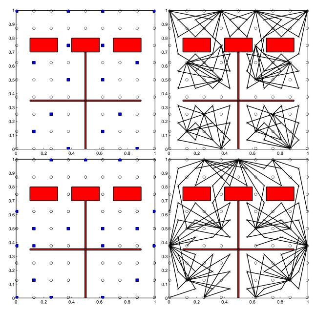
Fig. 9. **TOP ROW:** Placement obtained from the ILP solution. The figure on the left shows the selected cameras whereas the right figure shows the assignment of points (represented by  $\times$  symbols) in the workspace to the placed cameras. **BOTTOM ROW:** Placement obtained from the approximation algorithm. In this simulation, the ILP solution is 16 sensors whereas the approximation algorithm places 18 sensors.
