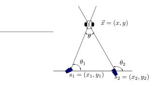
Fig. 1. The uncertainty in estimating the position of the target at x is given by:  $U(s_1,s_2,x)=\frac{d(s_1,x)\times d(s_2,x)}{\sin\theta}$
