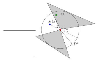
Fig. 7. The sensor  $s_2$  covers x because it satisfies the distance constraint and, together with  $s_1(x)$ , it satisfies the angle constraint as well.
