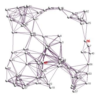
Figure 5: An example of the connectivity graph provided in iNSpect that was used to identify the variation in the number of neighbors throughout the network.
