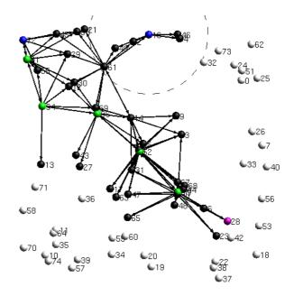
Figure 3: An example of the visualization window in iNSpect. In our protocols, we use black to identify nodes that intentionally drop packets, green are forwarding nodes, blue are sources, and purple are destinations.
