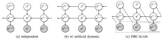
Fig. 2. Illustrations of three different assumptions on the dependencies of parameters for a simplified dynamic system that only has motion states  $\mathbf{x}^{\ell}$  and the corresponding sensor observations  $\mathbf{o}^{\ell}$ .
