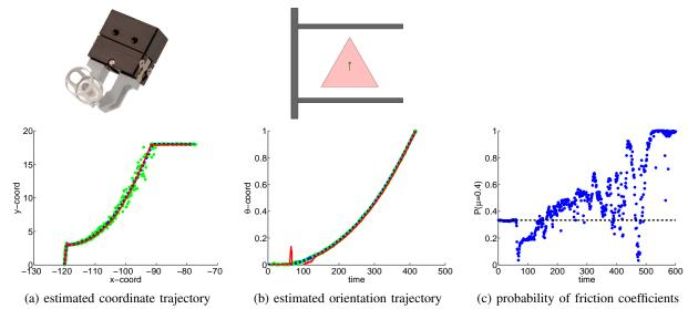
Fig. 4. (top left) A real parallel-jaw gripper and is simplification to the experiment of grasping a triangular object in the plane (top center). (bottom) Estimation results using a prototype implementation of DBC-SLAM. (a) Estimation of motion trajectories of the object's center of mass. (b) Estimation of orientation trajectory. (c) Estimation of the probabilities that the effective friction coefficient takes on it true values of 0.4.
