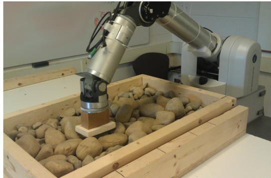
Fig. 1: Traction testbed with robotic foot.
