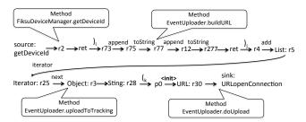
Figure 14: A source-sink path in Fiksu. When a flow is triggered by a library call, CFL-Explain labels the edge with the corresponding library method. When types change due to library calls, we show the new type at the target (e.g., List r5). We keep the identifiers exactly as they appear in the Jimple code.
