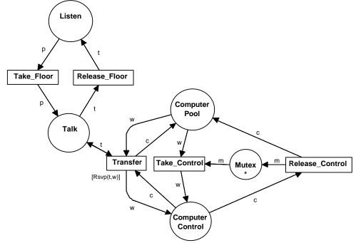
Figure 4. A session in which each participant has a presence in both the oral medium as a listener p or talker t and in the computer medium as a waiter w or controller c. Synergy is represented by the stipulation that a Transfer of computer control can occur only if the talker t receives an affirmative Rsvp from a participant w who is waiting to take control.
