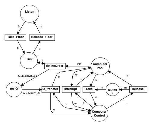
Figure 5. Discussion by t on the oral floor builds a queue Q of those waiting in the Computer Pool CP so that subsequent transfers of computer control may occur by the firing of the Q\_transfer transition when the controlling participant elects to make such a transfer.
