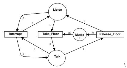
Figure 1(c). An oral meeting model in which there can be at most one speaker at a time and interruption is allowed.
