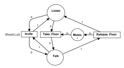
Figure 2. An oral meeting model in which the speaker t may invite another participant p from the listener place L to take the floor. The transition is guarded so as to be enabled to fire only if there is an affirmative Rsvp.
