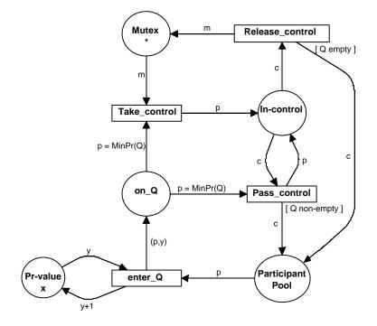
Figure 3. A floor control model incorporating a first come, first served protocol to be employed when the controller releases control and the queue of those wishing control is non-empty.
