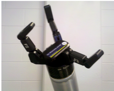
Figure 1.1: The Barrett Hand demonstrating two fingers spread apart, with the thumb shown on the right side of the image.
