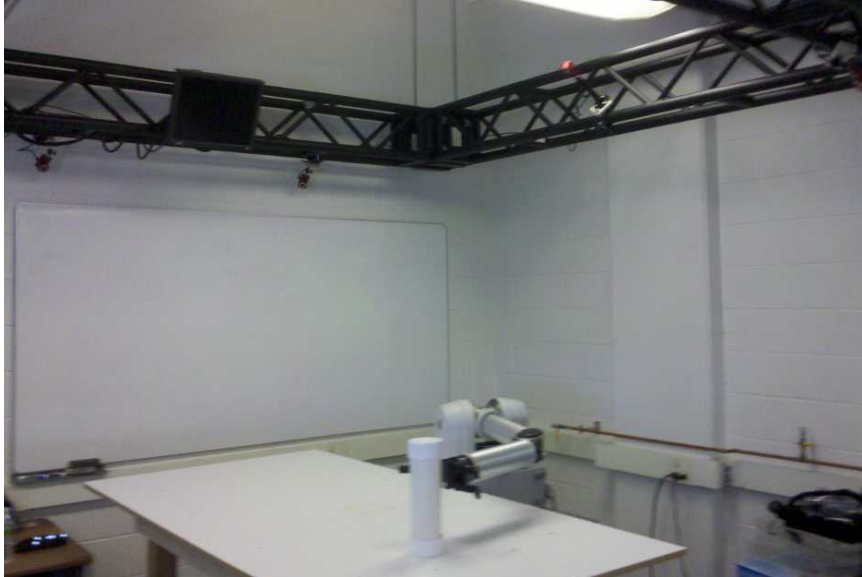
Figure 3.2: The experimental grasping test bed, showing both the Barrett Arm and Hand as well as the six-camera overhead tracking system by OptiTrack.
