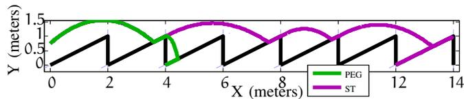
Fig. 4: Trajectories of the Polyhedral Exact Geometry and Stewart-Trinkle methods
