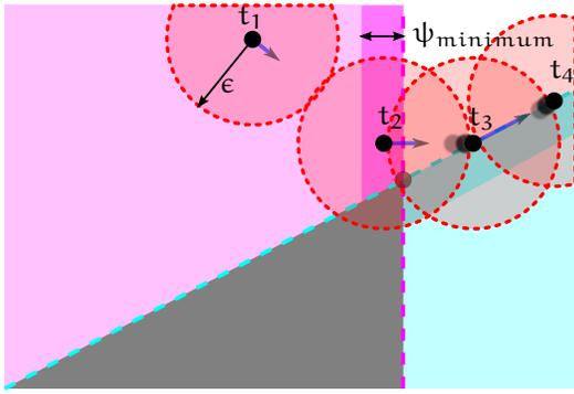
**Fig. 1:** Vertex at times  $t_1 \dots t_4$  moving within the constraint half-spaces near an object, Stewart-Trinkle method
