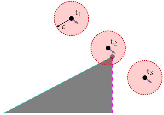
**Fig. 2:** Vertex at times  $t_1 \dots t_3$  moving in proximity to an object, Polyhedral Exact Geometry method
