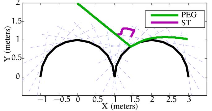
**Fig. 10:** Trajectories of the Polyhedral Exact Geometry and Stewart-Trinkle methods
