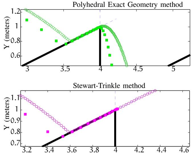
**Fig. 9:** Detailed view of trajectories of the Polyhedral Exact Geometry and Stewart-Trinkle methods under varying timesteps
