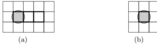
Fig. 7. The sizes of a mixer and a storage unit. (a) A mixer with 3 electrodes for droplets to move. S_{mix} = 15 . (b) A storage unit with 1 electrode for droplets to stay. S_{store} = 9 .
