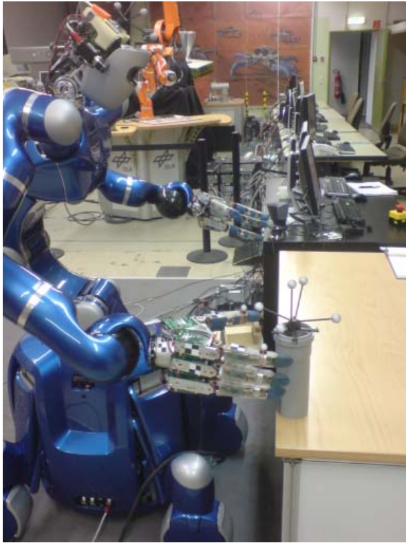
Fig. 3. DLR's humanoid Justin in front of a table. The task is to dynamically grasp the tube on the table.
