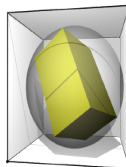
(c) Wrapping bounding sphere of a box with the AABB of the sphere
