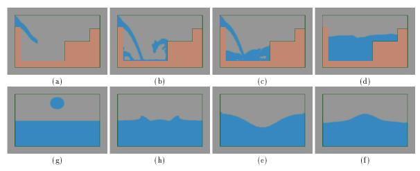
Figure 4: Frames from two dimensional animations making use of marker particles. A jet of water splashes into a concrete tank (a-d). A drop of water splashes into a shallow pool (e-h).
