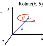
$$\begin{pmatrix} x' \\ y' \\ z' \\ 1 \end{pmatrix} = \begin{pmatrix} k_x k_x (1-c) + c & k_x k_y (1-c) - k_z s & k_x k_z (1-c) + k_y s & 0 \\ k_y k_x (1-c) + k_z s & k_y k_y (1-c) + c & k_y k_z (1-c) - k_x s & 0 \\ k_z k_x (1-c) - k_y s & k_z k_y (1-c) - k_x s & k_z k_z (1-c) + c & 0 \\ 0 & 0 & 0 & 1 \end{pmatrix} \begin{pmatrix} x \\ y \\ z \\ 1 \end{pmatrix}$$
