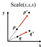
$$\begin{pmatrix} x' \\ y' \\ z' \\ 1 \end{pmatrix} = \begin{pmatrix} s_x & 0 & 0 & 0 \\ 0 & s_y & 0 & 0 \\ 0 & 0 & s_z & 0 \\ 0 & 0 & 0 & 1 \end{pmatrix} \begin{pmatrix} x \\ y \\ z \\ 1 \end{pmatrix}$$
