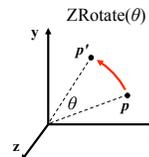
$$\begin{pmatrix} x' \\ y' \\ z' \\ 1 \end{pmatrix} = \begin{pmatrix} \cos \theta & -\sin \theta & 0 & 0 \\ \sin \theta & \cos \theta & 0 & 0 \\ 0 & 0 & 1 & 0 \\ 0 & 0 & 0 & 1 \end{pmatrix} \begin{pmatrix} x \\ y \\ z \\ 1 \end{pmatrix}$$
