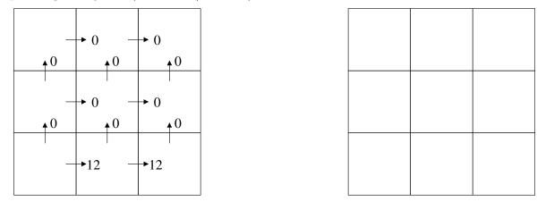
To model an incompressible fluid such as water, the divergence of each cell should be zero. In the cells below, fill in the velocities (left) and corresponding divergence (right) resulting after the *first iteration (or sweep)* of Foster & Metaxas' divergence correction from "Realistic Animation of Liquids". Note the direction of the velocities (use negative values if the flow travels in the reverse direction). Traverse the cells from left to right, top row first.
