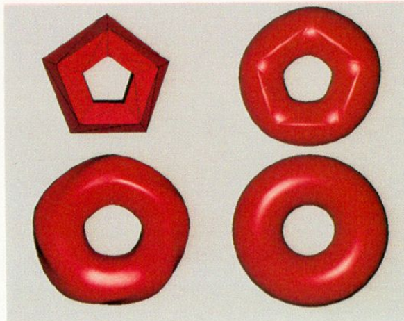
Figure 4: Interpolating a coarsely polygonized torus. Upper left: original mesh. Upper right: Shirman-Séquin interpolation[14]. Lower left: Interpolating Catmull-Clark surface. Lower right: Faired interpolating Catmull-Clark surface.
