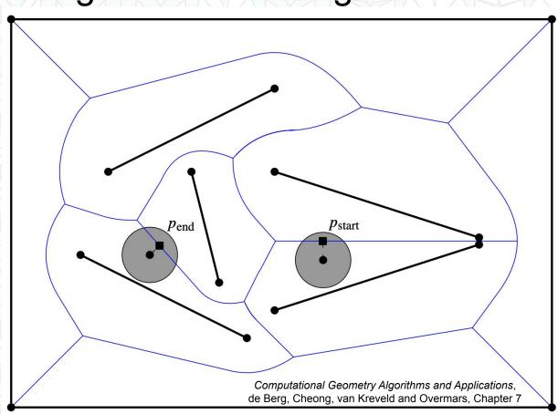
Let's move a circular/disk robot from the start position to the end position.
