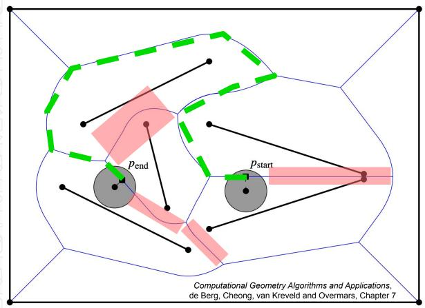
Step 3: Search the remaining graph for a connected path from start to end.
