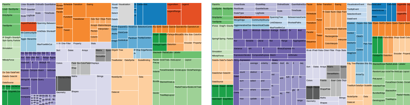
Fig. 2. Treemaps made with D3. The visualizations are implemented in pure HTML & CSS, improving browser compatibility. A stable layout algorithm enables animated transitions for changing cell values (from left to right) without disorienting rearrangements.
