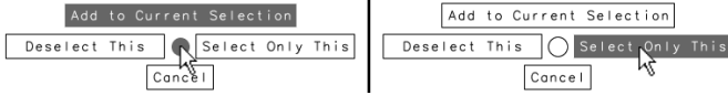
Fig. 8. The set operation menu. This menu appears immediately after a rectangle, lasso, or neighbourhood-radius has been input, effectively asking the user “what to do” with the nodes they’ve just specified. North, west, and east correspond to set union, set difference, and assignment, respectively. As with the other radial menus, the centre item corresponds to a default menu item, in this case the north item as indicated the co-hilting of north and centre. So, flicking up has the same effect as releasing over the centre with no dragging ( Top ). Flicking in other directions causes the centre to un-hilite ( Bottom ).
