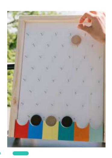
Disks are dropped from the top, hit the obstacles along the way, and eventually fall into one of the bins in the bottom.
