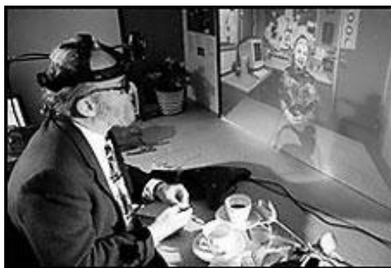
Figure 1. A local user on the left shares the same environment with a remote user on the right. A 3D description of the remote environment is projected stereoscopically on the screen from the viewpoint of the local user.
