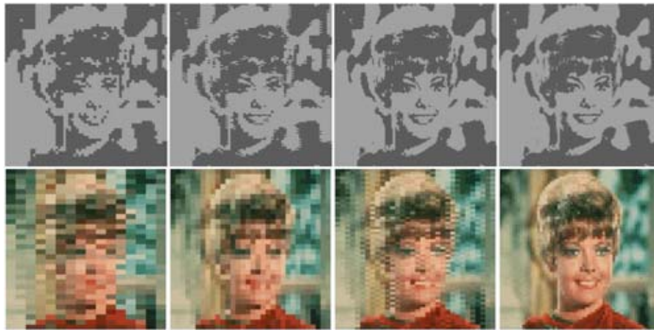
Fig. 13 “Zelda” under AS sequence (first row) and AC sequence (second row). Bit transmitted (from left to right): 0.78, 1.56, 3.12, and 6.25% of the color-mapped image size ( 256 \times 256 , 8-bit color map).
