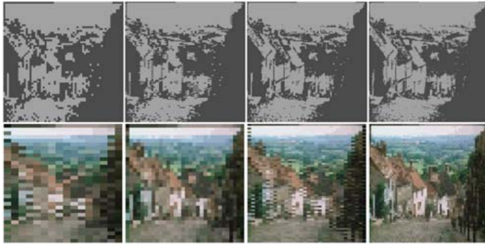
Fig. 11 “Goldhill” under AS sequence (first row) and AC sequence (second row). Bit transmitted (from left to right): 0.78, 1.56, 3.12, and 6.25% of the color-mapped image size ( 256 \times 256 , 8-bit color map).
