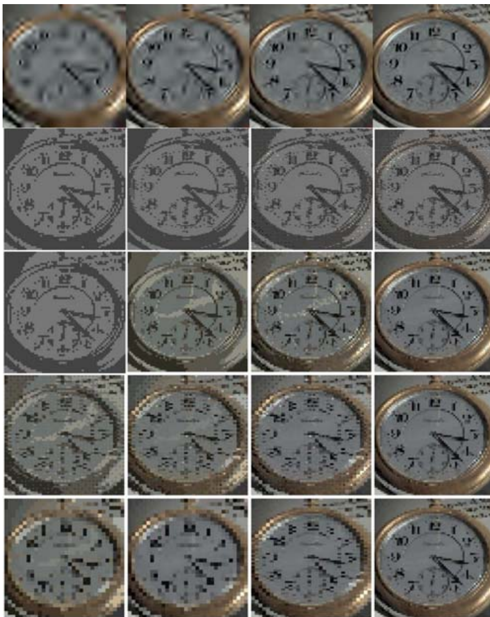
Fig. 18 “Watch” under SPIHT (first row) and SCPRC with [l, k] being [91,1] (second row); [64,2] (third row); [45,4] (fourth row); and [32,8] (fifth row). Bit transmitted (from left to right): 0.78, 1.56, 3.12, and 6.25% of the total bitstream size (SPIHT) or color-mapped image size ( 256 \times 256 , 8-bit color map) (SCPRC).
