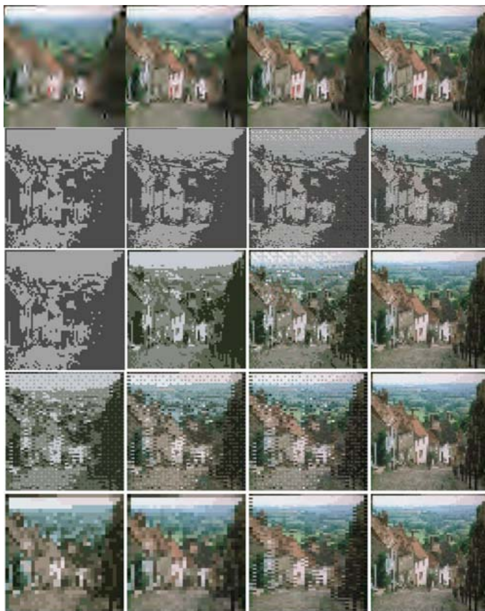
Fig. 17 “Goldhill” under SPIHT (first row) and SCPRC with [l, k] being [91, 1] (second row); [64, 2] (third row); [45, 4] (fourth row); and [32, 8] (fifth row). Bit transmitted (from left to right): 0.78, 1.56, 3.12, and 6.25% of the total bitstream size (SPIHT) or color-mapped image size ( 256 \times 256 , 8-bit color map) (SCPRC).
