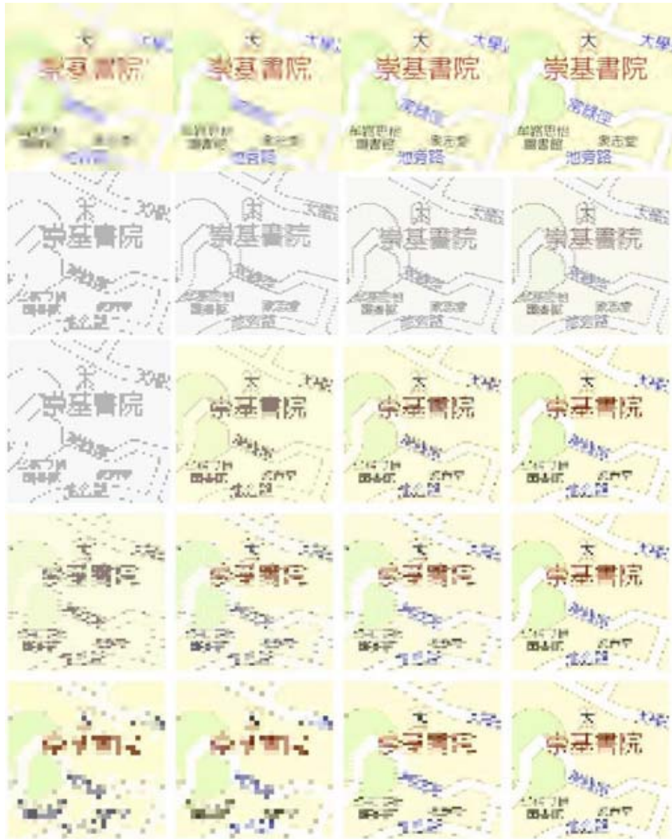
Fig. 16 “Map” under SPIHT (first row) and SCPRC with [l, k] being [91, 1] (second row); [64, 2] (third row); [45, 4] (fourth row); and [32, 8] (fifth row). Bit transmitted (from left to right): 0.78, 1.56, 3.12, and 6.25% of the total bitstream size (SPIHT) or color-mapped image size ( 256 \times 256 , 8-bit color map) (SCPRC).
