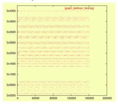
The plot shows the memory access pattern of the Bellman-Ford algorithm processing a directed graph with 1000 vertices and 4000 edges in the adjacency list representation (vecS, vecS). Only memory accesses to the graph data structure are drawn, and the addresses are shown relative to the smallest one. Red dots are distributed irregularly because edge vectors are allocated dynamically. The Bellman-Ford algorithm makes references to all edges at every
