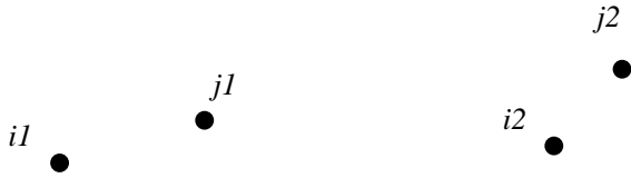
Fig. 4. The distance d_{ij} between the two compatible pairs [i1, i2] and [j1, j2] with coordinates [(x_{i1}, y_{i1}), (x_{i2}, y_{i2})] and [(x_{j1}, y_{j1}), (x_{j2}, y_{j2})] respectively, is \max(\alpha|x_{i1} - x_{j1}|, \alpha|x_{i2} - x_{j2}|, |y_{i1} - y_{j1}|, |y_{i2} - y_{j2}|) .
