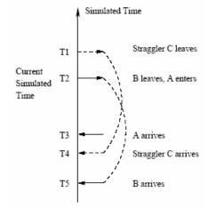
Figure 3: A Straggler Can Only Increase the Initial Position of Another at Entering the Service
