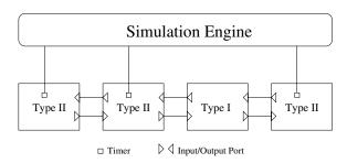
Figure 1: Simulation Engine for Type I and Type II Components
