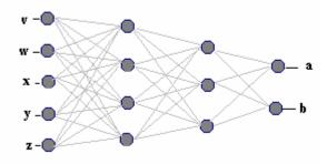
Figure 2 – Graphical representation of neurons interconnected receiving many inputs and produces 2 outputs
