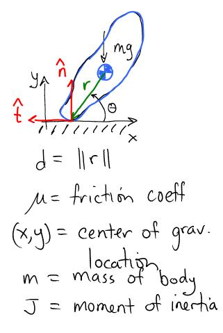
Write the instantaneous equations of motion in terms of  $\lambda_n$  and  $\Psi_n$ . The result should be an LCP of Size 1 in  $\lambda_n$ :  $0 \le \lambda_n \perp A \lambda_n + b \ge 0$
