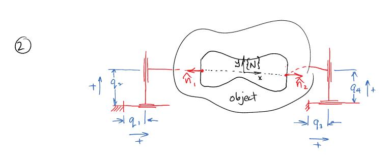
A hand with two fingers is grasping an object with contact points in a hole.
