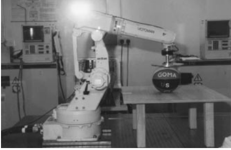
Figure 5: A flat fingertip rolling a ball on a plane
