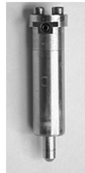
Figure 9. Photo of Pin Insertion Tool
