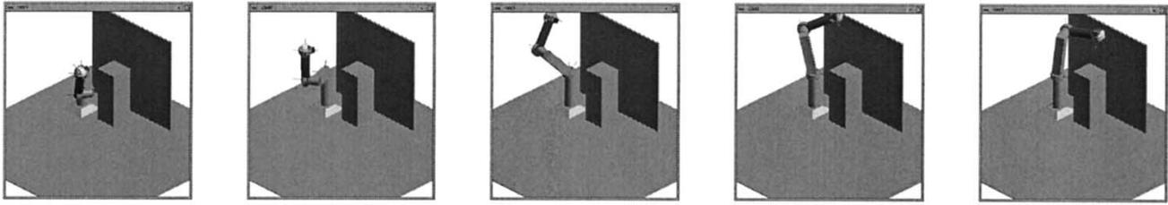
Fig. 12. Simulation snapshots of the 6-dof robot manipulator following the modified trajectory.
