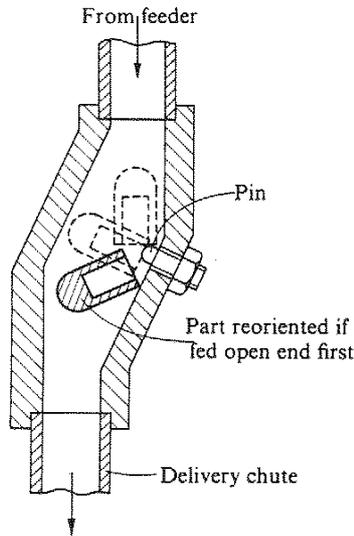
Figure 1: The exit orientation of the cup-shaped part must be with the curved portion down, regardless of the entering orientation [1].
