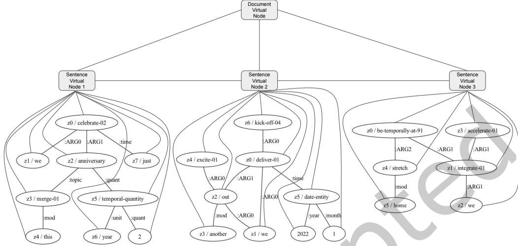
Fig. 4. An illustrative example of how sentence-level AMR graphs are aggregated into a document-level representation. The sentence-level AMR graphs (from left to right) represent the sentences: (1) We just celebrated the two-year anniversary of this merger. (2) We delivered another exciting outperformance in Q1 to kick off 2022. (3) We’re in the home stretch of our accelerated integration.
