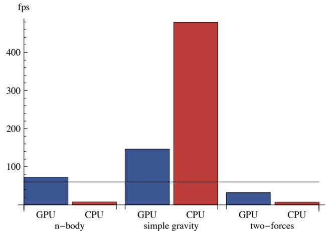
Figure 7: Simulation frame-rate of various different systems on CPU vs. GPU; higher values are better; the horizontal line rests at 60 fps
