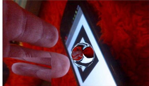
Despite the frustration caused by depth buffer rendering on a mobile device, reflection ended up producing moderately convincing results at interactive rates. Shader support and other updated features of GLES2.0 were successfully added to AndAR and they should be generally applicable to most meshes. Further work would hopefully get depth textures to render properly.
