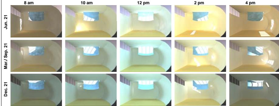
Using the standard CIE Sky Model [5], the system can render qualitatively accurate images. In designing the interesting curved geometry for the living space in this residential design, the architects are able to see the effect of the deflectors and windows. The curved diffuse blue deflector redirects the strong overhead noon sunshine from skylights, and additional windows on the western wall allow the warm late afternoon sun to penetrate deep into the room and wash over the far wall.
