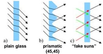
In a flat pane of glass, light rays are refracted, but exit parallel to the input rays. Light rays that pass through a prismatic panel are refracted differently and exit in two different directions due to the microfaceting. We can reverse engineer the directions of two "fake suns" allowing us to render the specular refractions efficiently.
