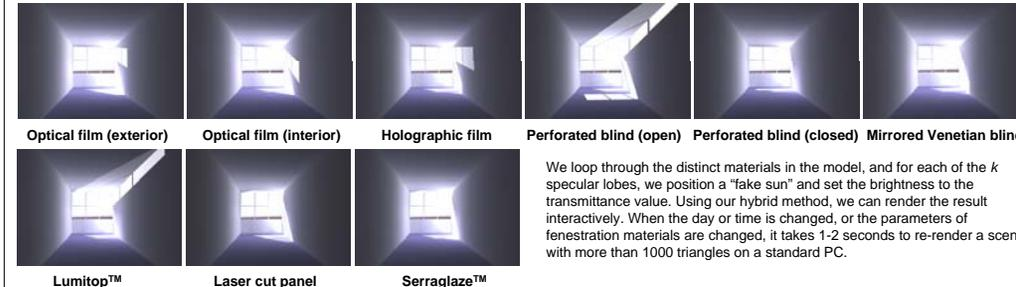
We loop through the distinct materials in the model, and for each of the  $k$  specular lobes, we position a "fake sun" and set the brightness to the transmittance value. Using our hybrid method, we can render the result interactively. When the day or time is changed, or the parameters of fenestration materials are changed, it takes 1-2 seconds to re-render a scene with more than 1000 triangles on a standard PC.
