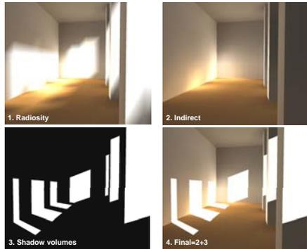
To achieve interactive rendering rates, we use a hybrid method of shadow volumes [3] for direct illumination and radiosity [4] for indirect illumination. We first calculate the indirect illumination, which is the difference between the first bounce initialization of radiosity and the final radiosity solution. Then we blend the direct illumination rendered by shadow volumes with the indirect illumination to generate the final result.
