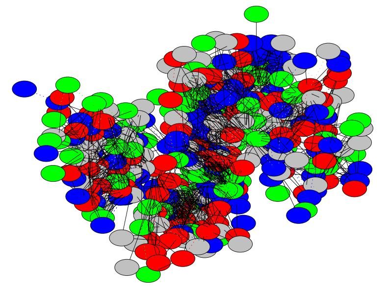
1.) Randomly initialize the partition. Solid lines indicate cut edges and dotted lines indicate intra-part edges.
