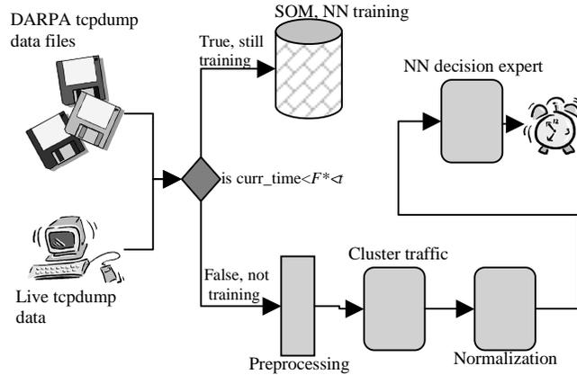
**Figure 1: System Architecture and Data Flow Diagram**
