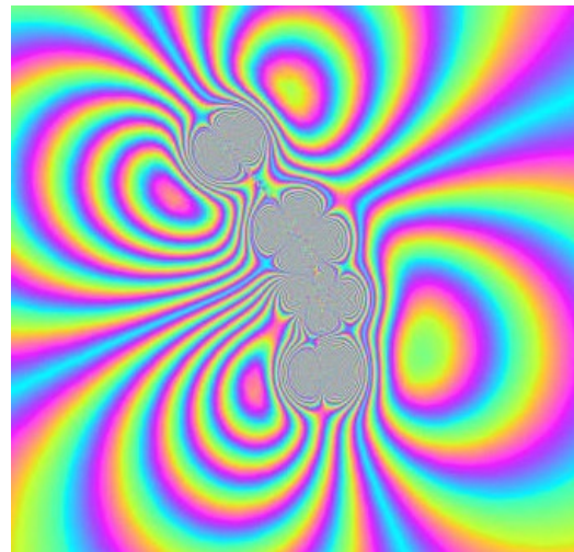
High Resolution: Use of PYRAMID for AMR dramatically improves InSAR fringe map over low-resolution case.
